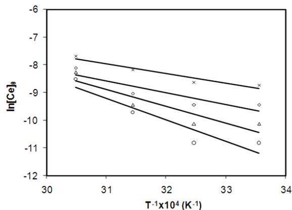
Fig. 12: Plot of  $\ln[Ce]_{\theta}$  vs.  $T^{-1}$  for Mn (II) biosorption onto P. Osreatus at pH 6.
