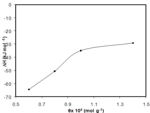
Fig. 13: Isosteric heat ( $\Delta H$ ) as a function of surface coverage  $[\theta]$  for Mn (II) biosorption onto P.Ostreatus.
