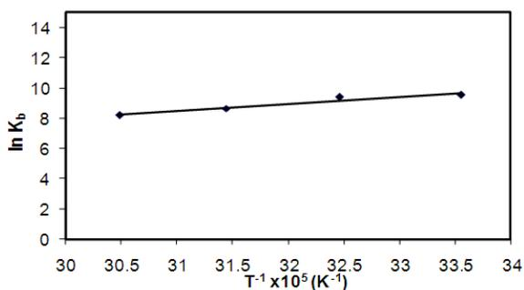
Fig. 11: Plot of  $\ln K_b$  vs.  $1/T$  for biosorption of Mn (II) by *P.Ostreatus* at pH 6.
