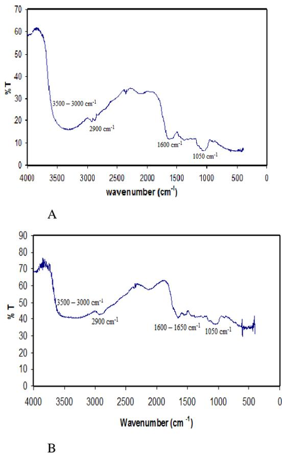
Fig. 4: FTIR spectra of P. Ostreatus (A) before (B) after sorption of Mn (II).
