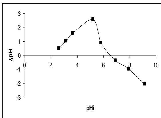
Fig. 5: Point of zero charge (PZC) of P. Ostreatus at 298 K.
