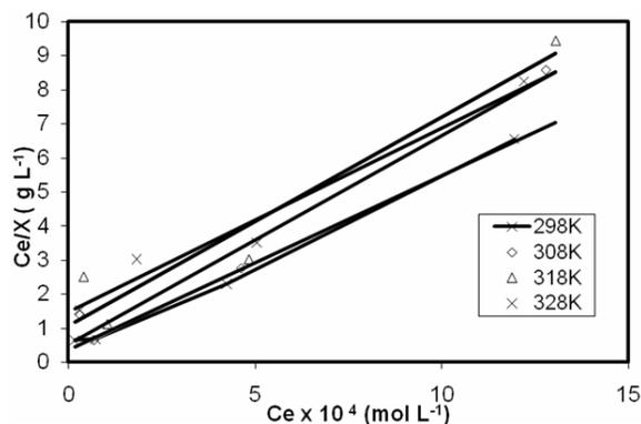
Fig. 10: Langmuir plots for Mn (II) biosorption by P. Ostreatus at different temperatures and at pH 6.
