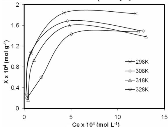
Fig. 9: Effect of temperature on Mn (II) biosorption by P. Ostreatus at different temperatures and at pH 6.
