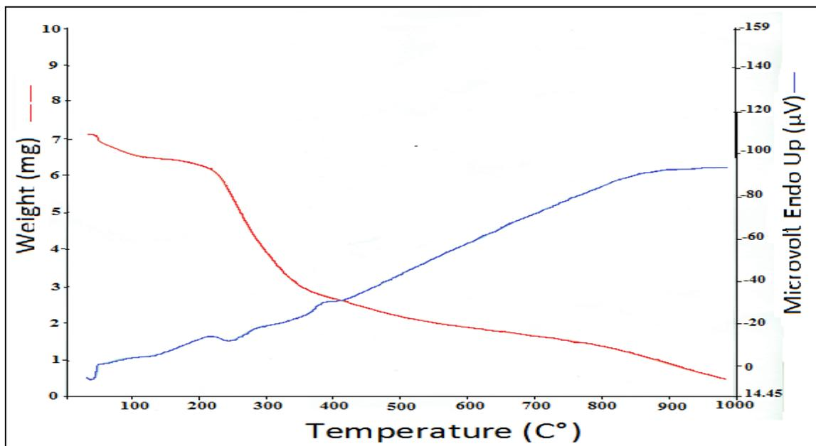
Fig. 3: Thermogravimetric / Differential thermal analysis of P. Ostreatus.
