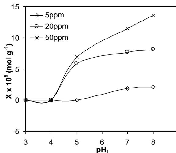
Fig. 8: Effect of pH on Mn (II) biosorption by P. Ostreatus at 298 K.
